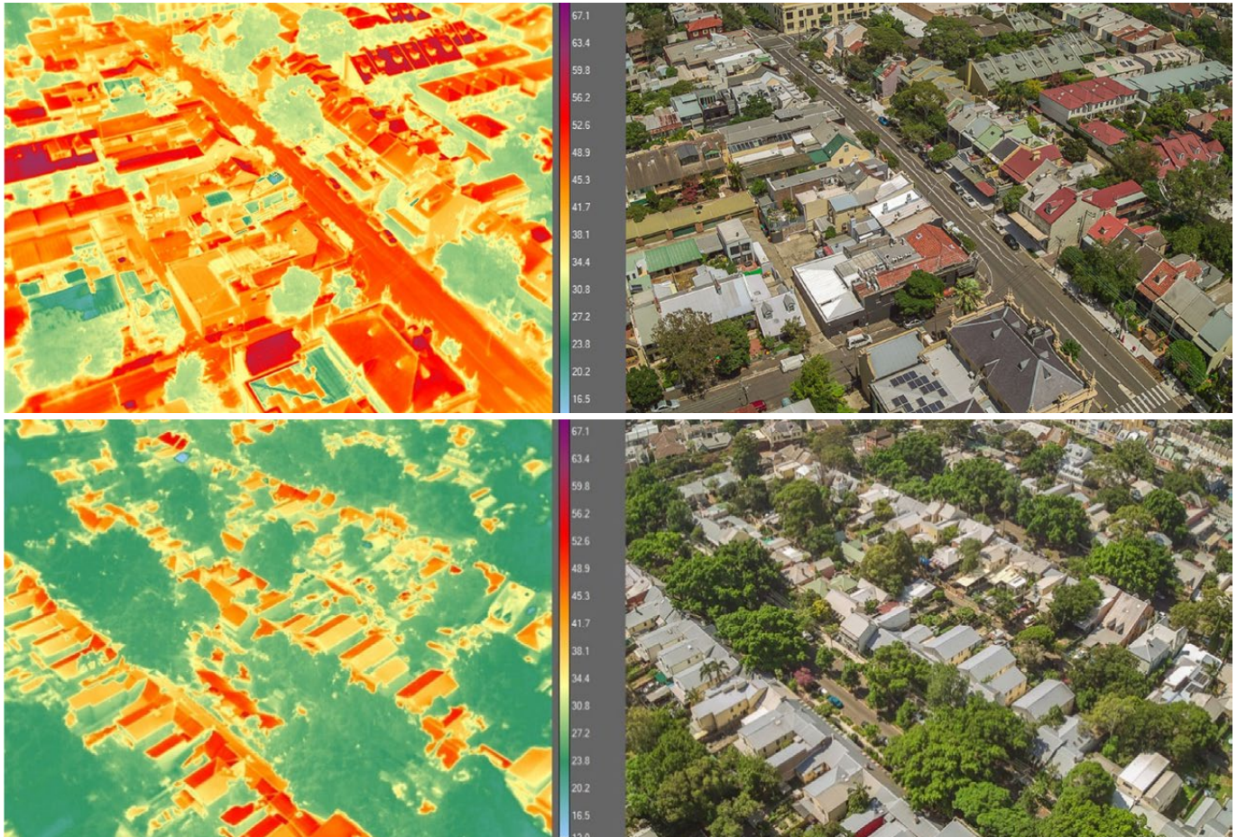
Figure 36: Thermal mapping of two areas over Glebe in January 2019 illustrating the reductions in temperature and substantial cooling benefits of trees and urban canopy cover. The upper image over St Johns Rd, the lower image indicating nearby and well treed Westmoreland St. (Source: City of Sydney Greening Strategy 2023)
