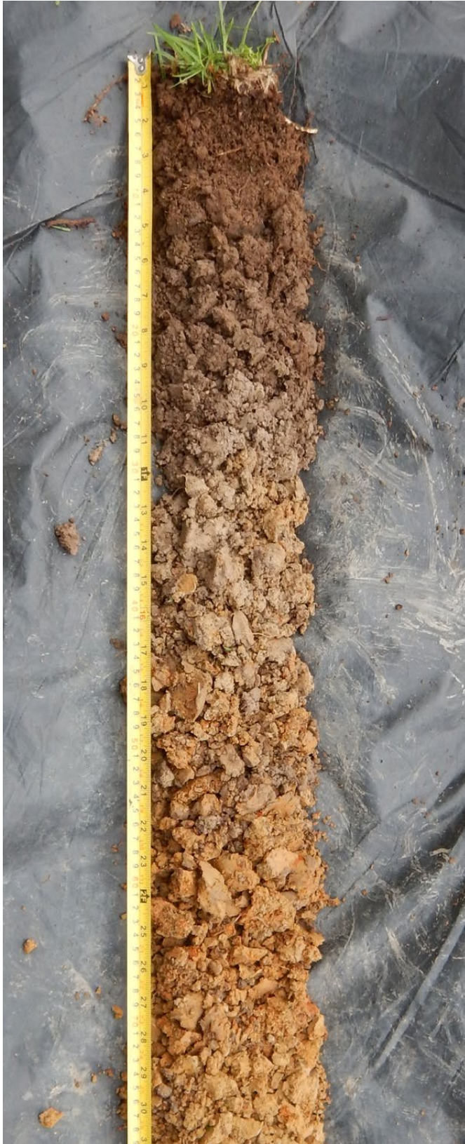
Figure 50: Typical soil profile from the clay and shale based soils of the Cumberland Plain. (Source: Arterra)
