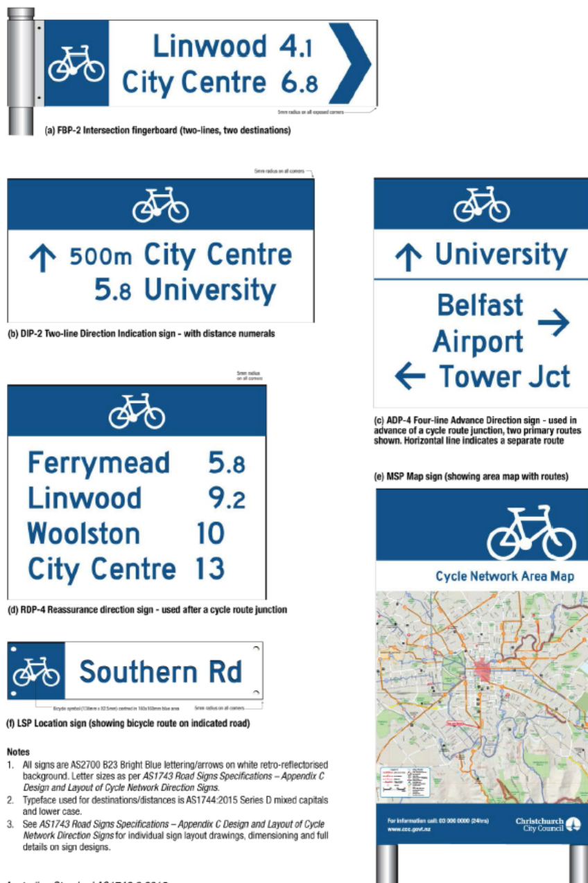
Veloway and primary cycle route directional sign family – general sign types and layouts
