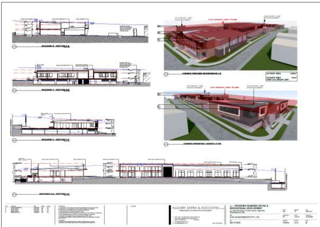
Figure 6: Perspectives and sections showing the area of non-compliance (areas of non-compliance shaded). Source: P.4343 Sheet A12 Rev E prepared by Algorry Zappia and Associates.
