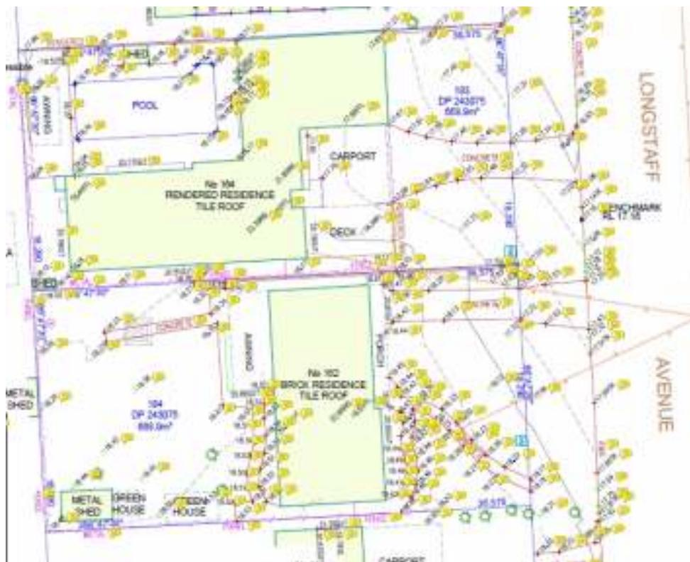
Figure 3: Contour and Detail Survey Plan (Source: Ensure Consulting Pty. Ltd, Rev. A, Drawing No. 200139 DE-01, dated 2/09/2019)
