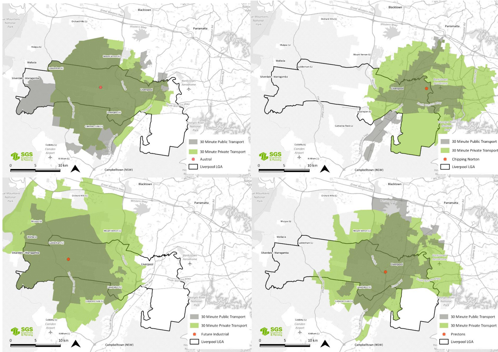
FIGURE 40: THE 30 MINUTE TRAVEL CATCHMENTS BY PUBLIC AND PRIVATE TRANSPORT OF FOUR INDUSTRIAL PRECINCTS WITHIN LIVERPOOL LGA
