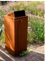
Figure 6.308 Slim box bins made from untreated corten steel.
