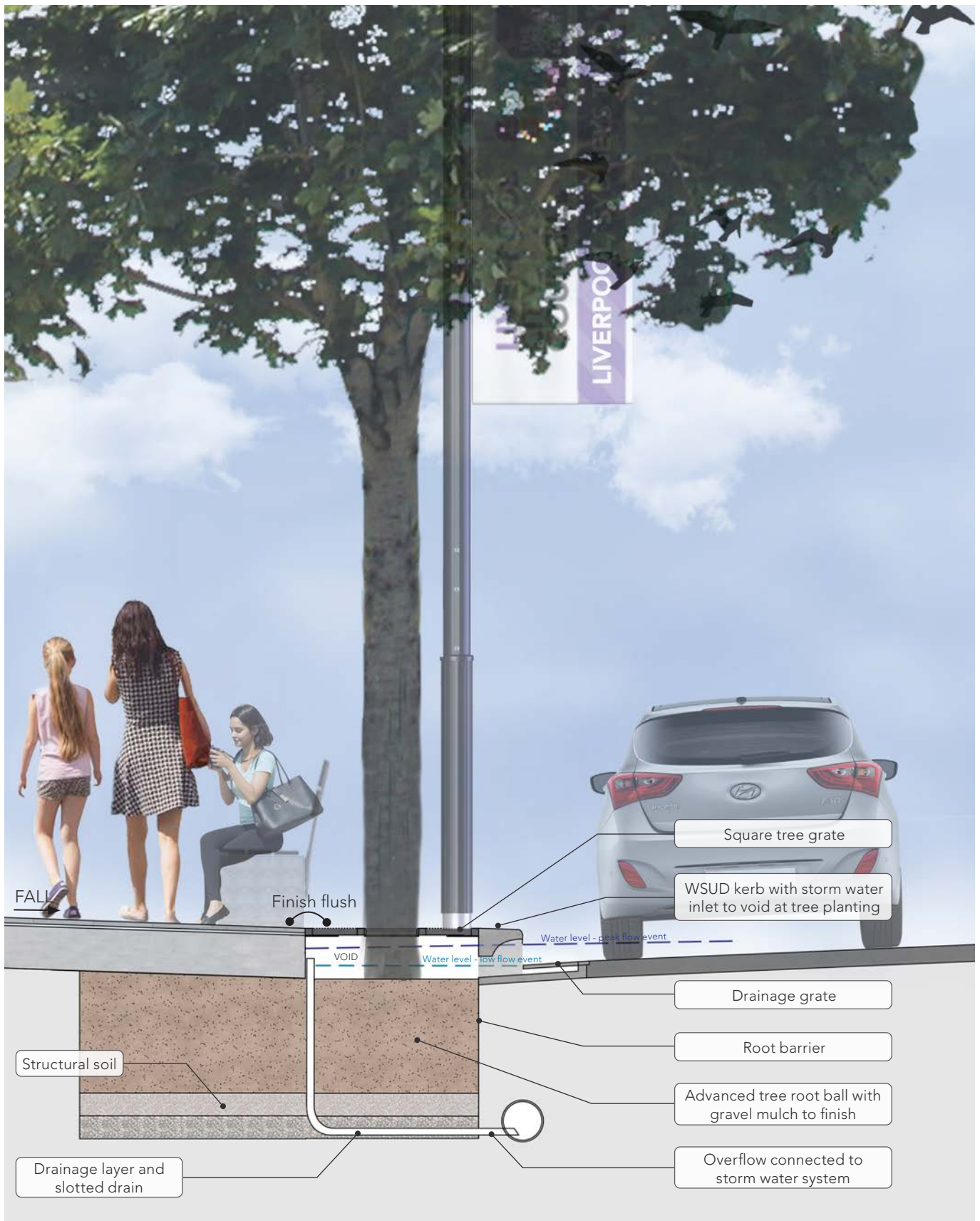
Figure 6.245 WSUD Tree Pit Detail (Liverpool City Council)
