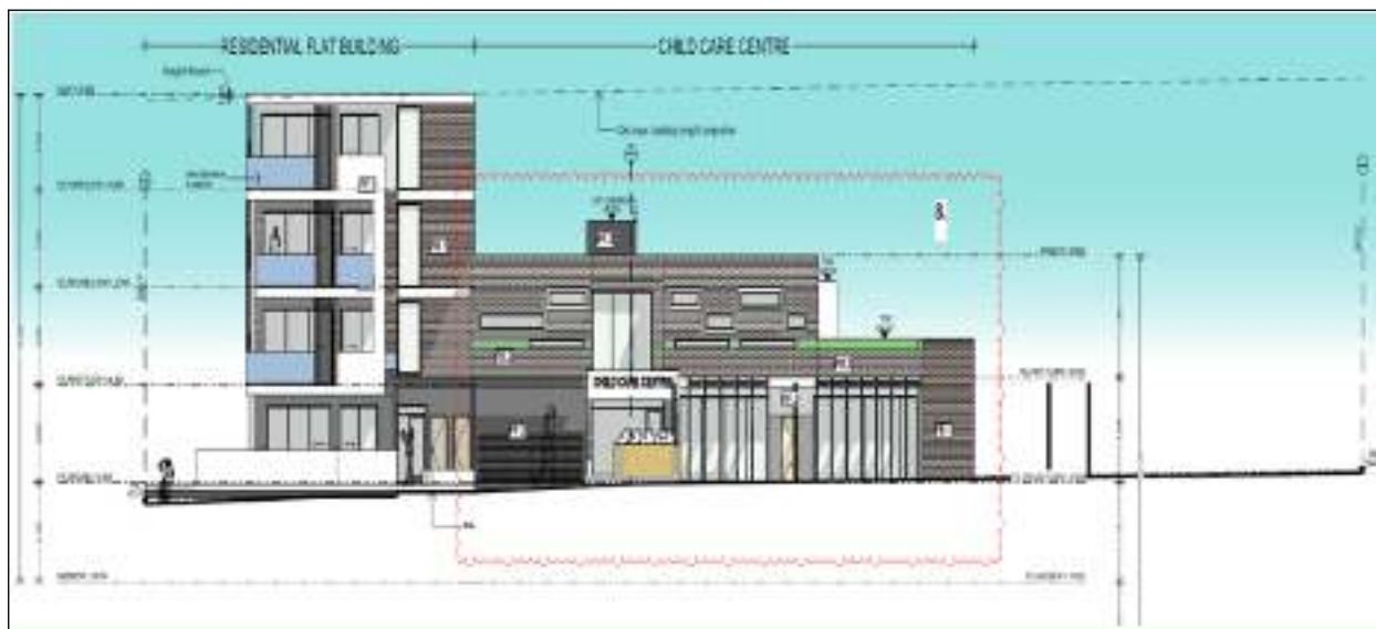
Figure 8: Height plan study/front elevation submitted with Clause 4.6 variation. (Maximum building height of 12m shown in dashed line) (Source: Clause 4.6 variation prepared by Think Planners).
