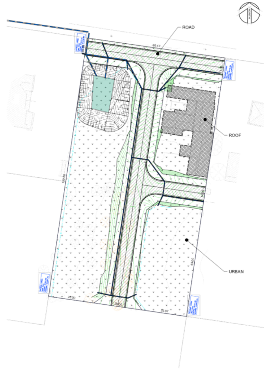
PROPOSED WATER QUALITY CATCHMENT PLAN SCALE 1:500
