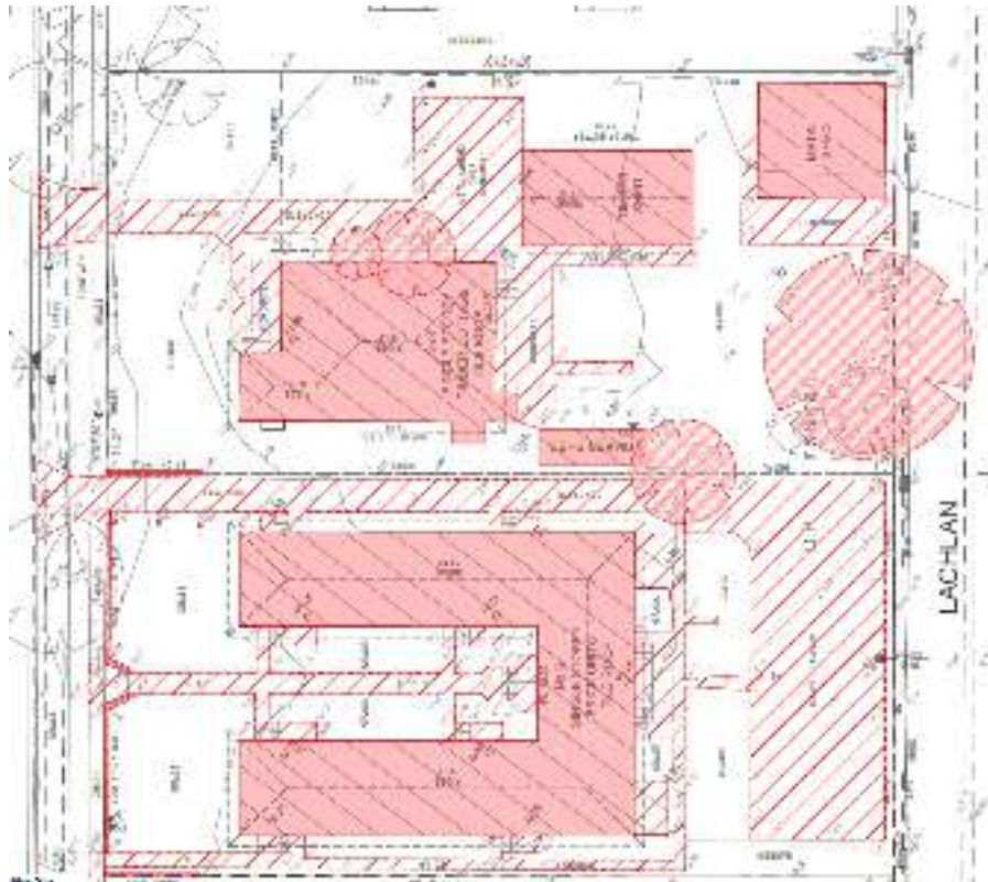
Figure 8: Demolition and Tree Removal Plan (Source: Zhinar Architects Pty. Ltd., Ref. 08632, Rev. C, dated 12/06/2020)
