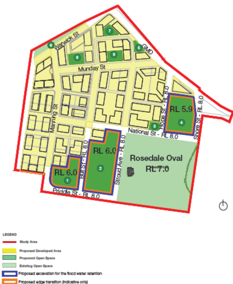
Figure 3: Proposed open space areas, including those indicated for flood water retention bounded in purple. Source: Conybeare Morrison International
