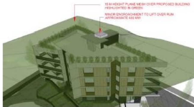
Figure 1 Diagram Indicating the 15m height plane over the proposed development and extent of proposed height variation.
