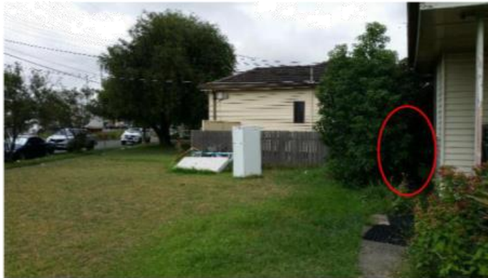
Figure B2 Noise logger installed at front boundary of the site
